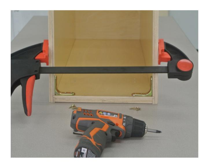
Screw back panel to bottom panel using 1" screws into the pre-drilled holes.
