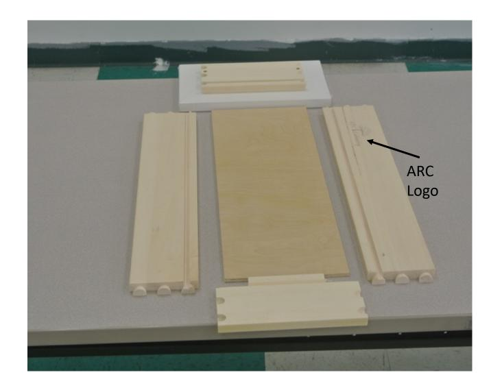
Assemble drawer with dovetail joints. ARC Cabinetry logo should be closer to drawer face.
