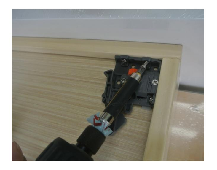
Slide latches as attached on the bottom of drawer.
