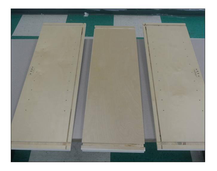
Clamp the cabinet sides with the top and bottom panels as shown. Ensure proper fitting in all dado grooves.
