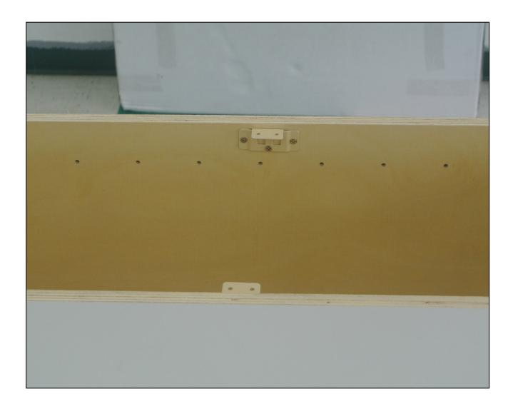
Place face frame on the box ensuring proper fitting on all dado grooves.
