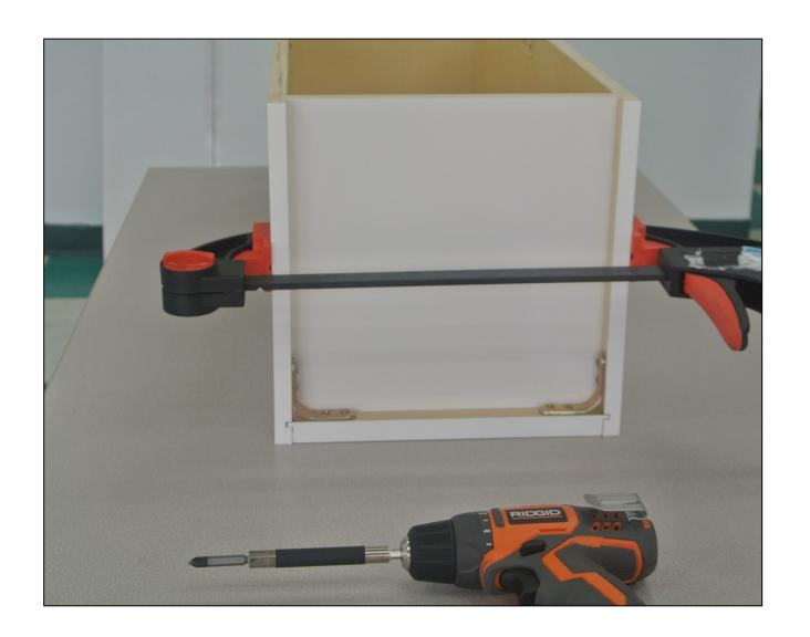
Screw back panel to top and bottom panel using 1" screws into the pre-drilled holes.
